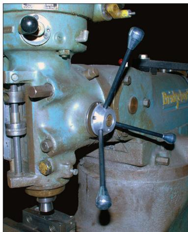
Sturdy construction features a solid aluminum machined center (not a casting), with a 1" bore and a 3" diameter. (3) heavy duty solid steel spokes and knobs extend approx. 6-1/2" from center. Plated finish. Made in USA.
