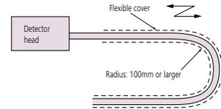
**Note)** It is important to ensure that the signal cable does not interfere with, and is not chafed by, any part of the machine.
