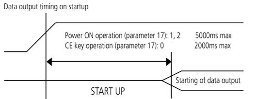
The display mode at startup can be selected with the parameter (KA-200 Counter).
