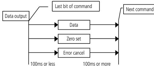
Each value in the timing chart indicates response time to a command. Consequently, be aware that this command may cause a difference between a detected point and the actual one when the slider is moving.
